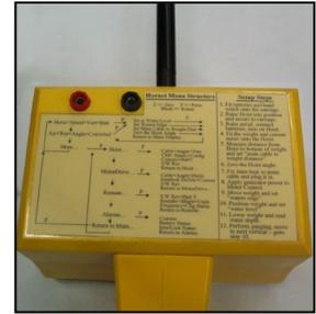
The two main menus show the most used information. Pressing the scroll menu knob while in these menus allow zero functions to be performed. Stepping into the More... menu allows data specific to the Hoist, Drive Control, Remote Control and Alarms to be displayed.
