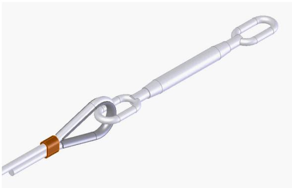
Slide the swage over the looped cable and crimp it
