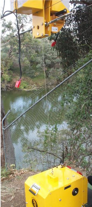
Lift the Hoist using the manual winch
