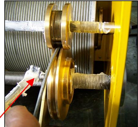
Grease the Hoist sheave shaft.
