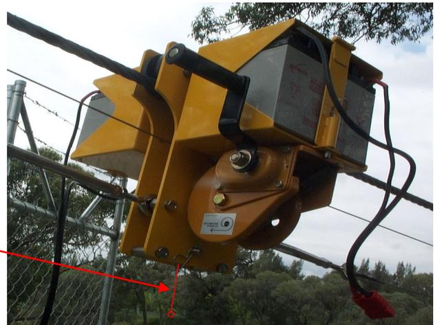
Hook the cable to the hoist as shown
