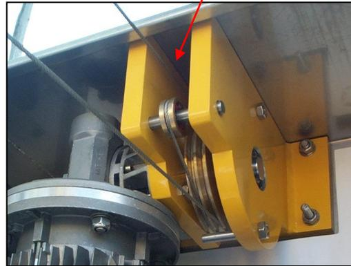
Keep running the cable till you get to the operating side. Feed the cable from the top as shown.
