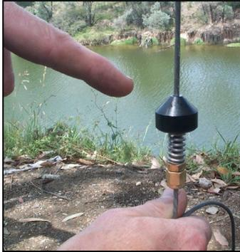
The hoist cable has a conical device clamped near the end of the cable. As the hoist cable is almost completely wound in, the conical device on the cable will press onto the rollers, causing a limit switch to stop the hoist. This prevents the hoist from self-destructing if it is wound up too far. A limit switch is also operated if the cable is let out too far. This will stop the drum with about 3 wraps remaining, to hold the heaviest weight used.
