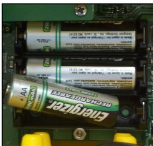
In an **emergency** you can use 3 x AA Alkaline batteries to power the Remote Control. Simply remove the 4 screws that secure the front panel of the Remote Control, then remove the lower screw on the strap over the 3 batteries and rotate the strap out of the way. Replace the 3 x NiMh batteries with 3 x alkaline batteries and re-assemble the Remote Control.
