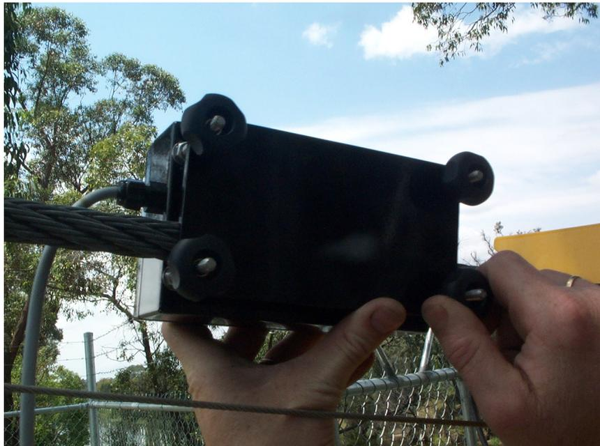
When tightening the knobs, make sure that the cable is in contact with the two lower studs (so that the box is aligned with the cable). This allows the internal inclinometer to measure the cable angle.
