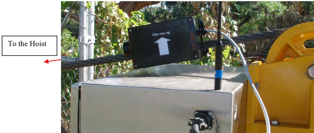
The Drive Control Interlock Box also contains an Inclinometer to measure the angle of the main cable which will allow the true horizontal distance across the river to be automatically calculated.
